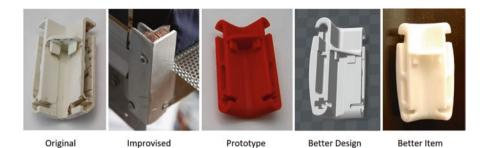
Fig. 14.1 3D-printed corner brackets printed by Field Ready
